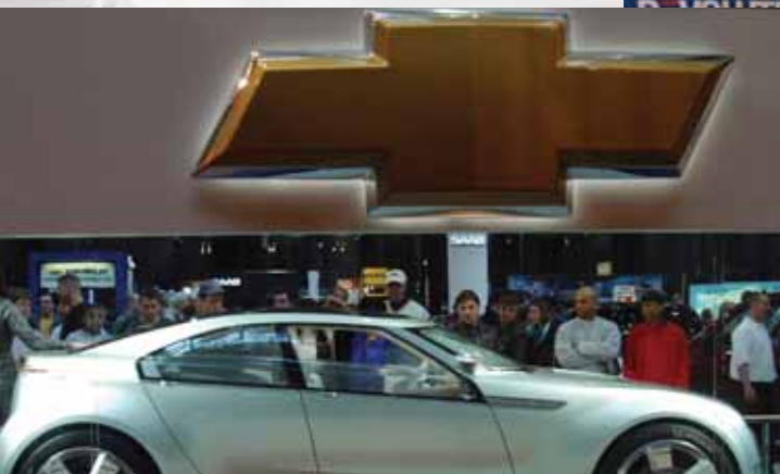
The Chevrolet Volt concept is built on a platform called E-flex. The Volt is a lithium-ion battery-powered electric car with a range of 40 miles in the city after a six-hour charge.
