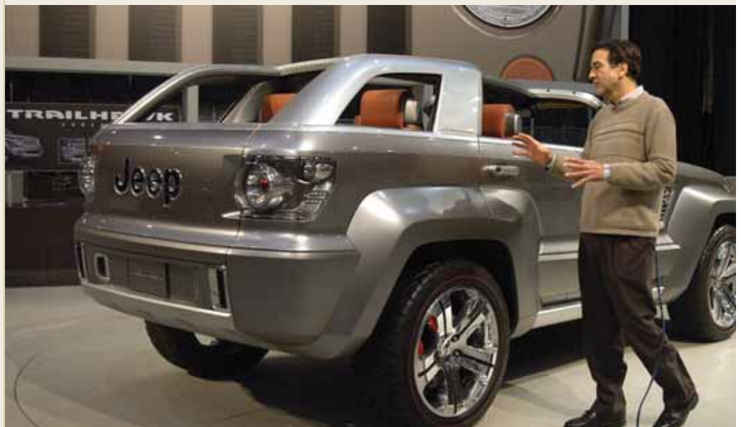
Scott Newell, anchor/reporter features the Jeep Trailhawk concept during WKYC's (NBC) morning show "Channel 3 News" on Saturday, March 3. The Trailhawk is built on a Wrangler chassis and allows open-air trekking with roll-down quarter-panel glass and a removable glass roof.
