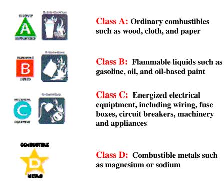
Remember that the extinguisher must be appropriate for the type of fire being fought. Multipurpose fire extinguishers, labeled ABC, may be used on all three classes of fire. If you use the wrong type of extinguisher, you can endanger yourself and make the fire worse. It is also very dangerous to use water or an extinguisher labeled only for Class A fires on a cooking-grease or electrical fire.
