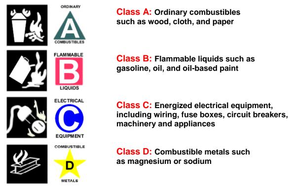
Remember that the extinguisher must be appropriate for the type of fire being fought. Multipurpose fire extinguishers, labeled ABC, may be used on all three classes of fire. If you use the wrong type of extinguisher, you can endanger yourself and make the fire worse. It is also very dangerous to use water or an extinguisher labeled only for Class A fires on a cookinggrease or electrical fire.
